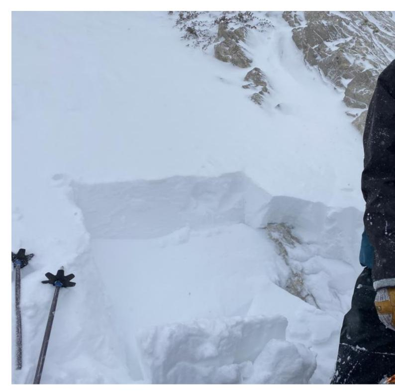
From obs 11/11/21: "Dug a snow pit at 8,280ft adjacent to a chute. It was NW aspect. We found a ~35cm 1 finger windslab sitting on top of a ~25cm knife hard slab. We got CT 12 on the first slab and CT 15 on the deeper slab. On the ECT, we got a slight fracture at 15 taps and a full fracture at 17 (ECTP+2). This layer seemed to be on all aspects we looked at above tree line on NW faces. Bellow treeline, the snowpack was shallower and seem to lack these slabs." Photo: J. Krause
