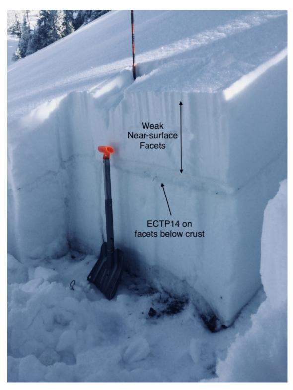
We found unstable test results on weak facets below the Thanksgiving crust on the west side of the Bridger Range. WNW aspect at 8100'. This instability is not widespread, but worth digging to look for before riding steep terrain. We found mostly stable conditions on slightly different slopes nearby. Weak, sugary facets above the crust will be the main concern when more snow falls. Photo: GNFAC
